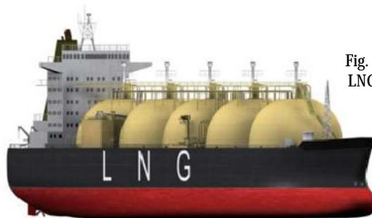
Fig. 1. Moss-type LNG carrier [10]
